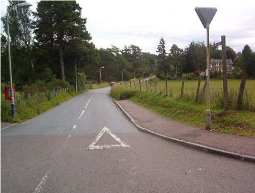
Fig 5 Station Road showing road to be re-positioned further right to improve visibility at junction with Perth Road.
